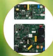
PCB for brush AC motor PCB for brushless DC motor
